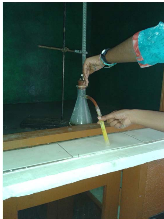
Figure 2. Bench-top hydrogen sulfide gas generator is being used in the laboratory for precipitating cadmium sulfide
