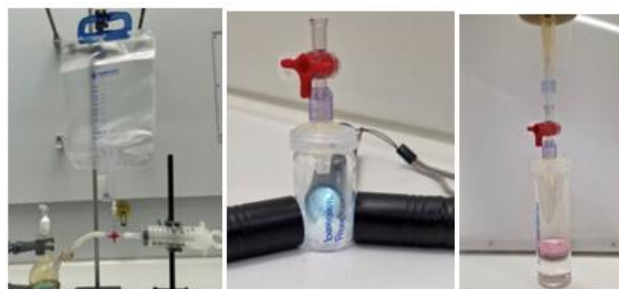
Figure 4. Set-ups of the experimental steps: Step 1: Evolution of nitrous fumes, Step 2: Irradiation with UV-light in the presence of the photocatalyst (three UV-flashlights), Step 3: Transfer of a gas portion into a vial filled with Griess reagent via a syringe (Pictures: Lisa Schnödewind).
