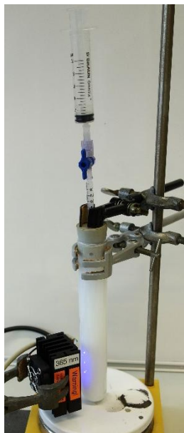
Figure 7. Compact set-up for photoreforming ethanol.
