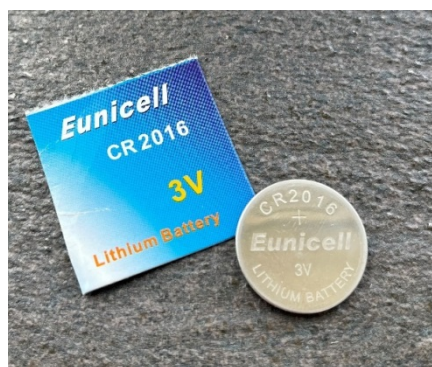
Figure 1. Representation of a lithium-manganese dioxide battery (button cell - own picture taking)
