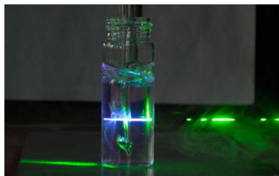
Figure 3. Photon up-conversion from green to blue - Anti-Stokes Shift (photograph by Nico Meuter )
