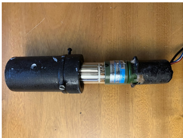
Figure 2. Photomultiplier with socket (right) and housing (left).
