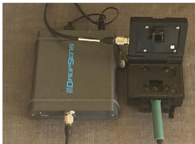
Figure 3. Experimental setup used. Potentiostat and ECL cell with photodiode
