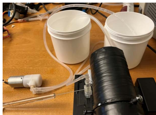
Figure 15. Injection of \text{H}_2\text{O}_2 with a Hamilton syringe (25 \mu\text{L} ) into a continuous fresh luminol solution. Left: peristaltic pump, top: storage vessel for the luminol solution and waste bin
