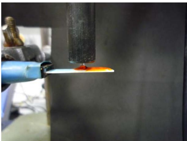
Figure 3. Detail of Figure 2: Electrode, glass fiber, housing for the fiber
