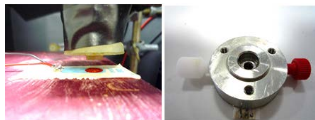
Figure 1. Left: Screen-printed electrodes with photomultiplier tube. Right: Modified ECL cell; at the bottom of the cell are the screen-printed electrodes
