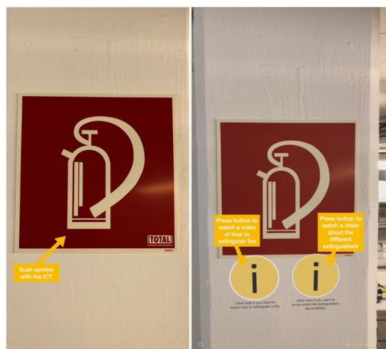
Figure 5. Extinguisher Symbol without (l.) and with (r.) Augmented Reality
