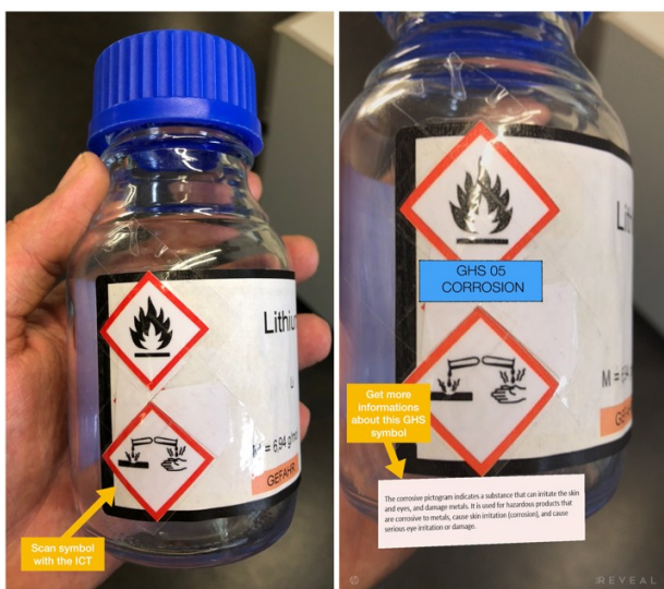
Figure 9. GHS Symbols without (l.) and with (r.) Augmented Reality
