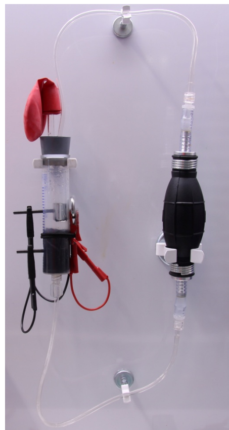
Figure 13. Experimental setup of the hybrid flow battery "to go" with a scrunchy
