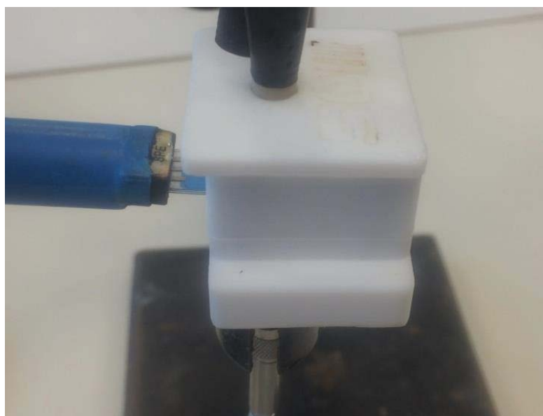
Figure S8. Electrochemical cell (white). Top: Excitation fiber (connected with the light source), read fiber (connected with the spectrometer). Bottom: Transmission fiber (connected with the spectrometer). Left: SPE with electrode holder (blue).
