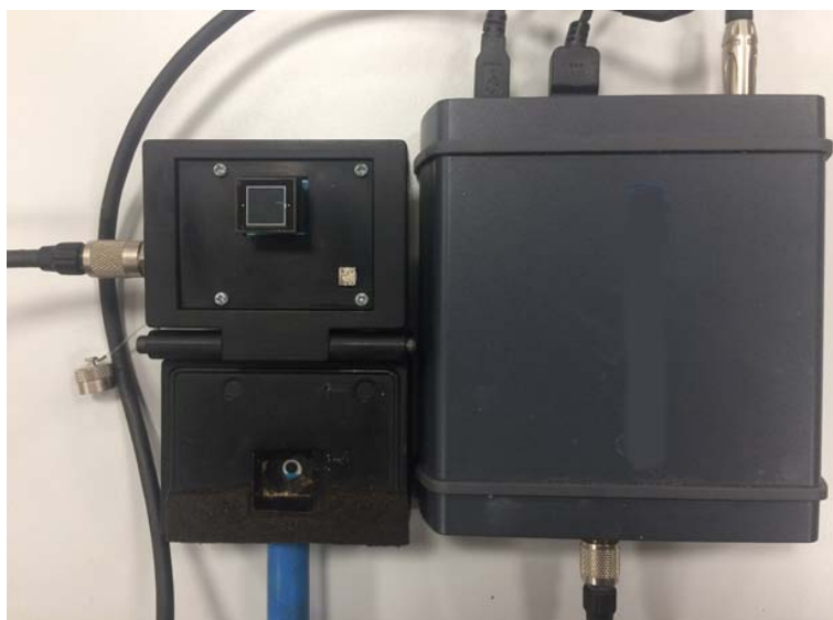
Figure S11. ECL-Stat from DropSens. Left: Chamber with SPE, above: photodiode. Right: potentiostat.
