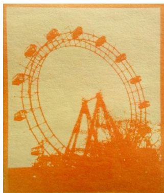
Figure 17. Diazotype with a mixture of a yellow and a red azo dye (motif: Giant Ferris Wheel in the Vienna Prater/Austria)
