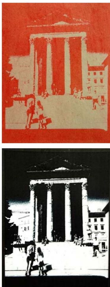
Figure 15. Top: Diazotype with a red azo dye (motif: Temple of Augustus, Pula/Croatia); bottom: Foil print used.
