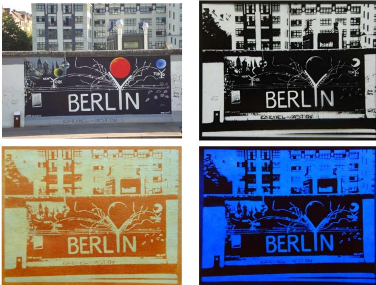
Figure 13. From top to bottom: Original photo (Ducci), printout as black and white image on foil, image obtained by diazotype, same image under UV light (motif: East Side Gallery Berlin/Germany)
