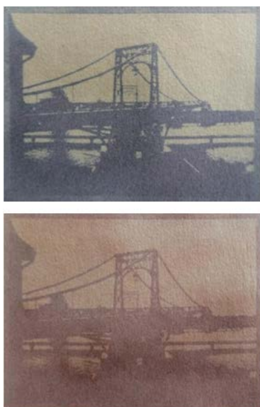
Figure 19. Diazotype with a blue azo dye (top), which takes on a reddish-brown hue at a lower pH value (outgassing of ammonia) (motif: Kaiser Wilhelm Bridge, Wilhelmshaven/Germany)
