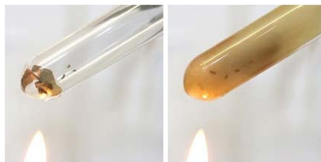
Figure 7. Thermolysis of 5-diazosalicylic acid. The time between the two images was 1/25 s. (Photographs: Ducci)
