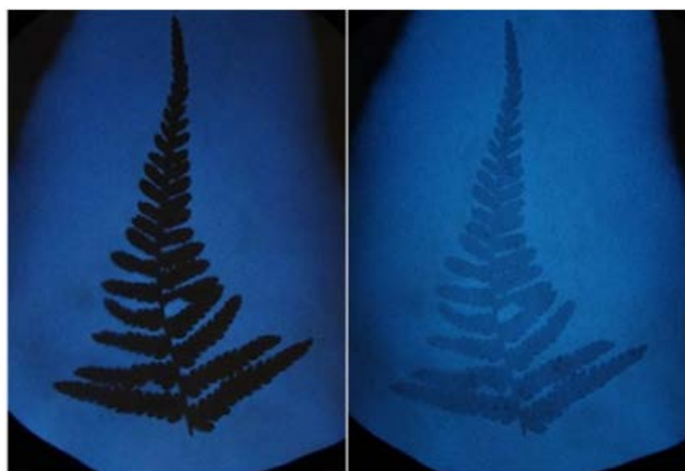
Figure 10. Left: Photochemically generated image using a fern leaf under UV light. Right: The same image after prolonged irradiation with UV light ( \lambda = 365 \text{ nm} ). (Photographs: Ducci)
