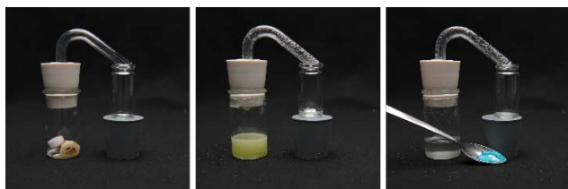
Figure 7. Observations during the decomposition of a UHP tablet by molybdate. The resulting water vapour is transferred and detected with anhydrous copper sulphate.
