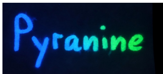
Figure 14. Ammonia gas sweeping from right to left over a writing made of acid pyranine solution, which is invisible in daylight. (Photograph: Ducci)
