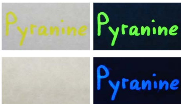
Figure 12. The colour solution of a yellow highlighter (top left) containing pyranine fluoresces intensely green under UV light (top right). It can be made invisible by hydrochloric acid (bottom left). Under UV light, the invisible writing fluoresces intensely blue (bottom right). (Photographs: Ducci)
