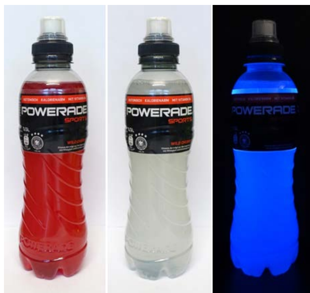
Figure 10. Reductive cleavage of azorubine in Powerade Wild Cherry using a fabric colour remover containing sodium dithionite. Left: Powerade Wild Cherry, middle: after addition of the colour remover, right: the bottle from the middle under UV light. (Photographs: Ducci)
