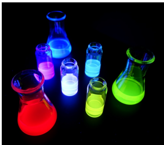
Figure 5. Demonstration of additive colour mixing with fluorescent solutions. In the Erlenmeyer flasks, the solutions fluoresce in the three primary colours. The rolled rim vials contain the mixtures. (Photograph: Ducci)
