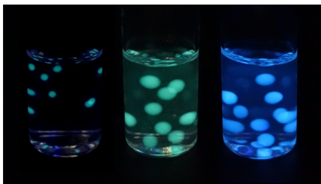
Figure 15. The alginate beads loaded with fluorescent indicators exhibit a different fluorescent behaviour in the acidic (left), neutral (middle) and alkaline (right) solution. The photograph was taken shortly before the fluorescence in the left vial completely extinguished. (Photograph: Ducci)
