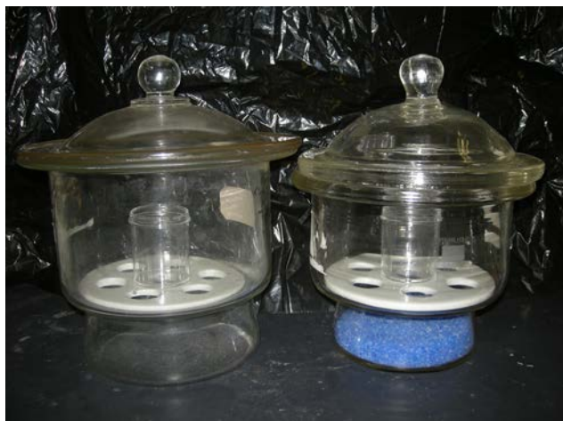
Figure 19. Use of desiccators in lieu of a glove box
