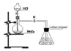
Figure 2. The apparatus was used to prepare chlorine gas
