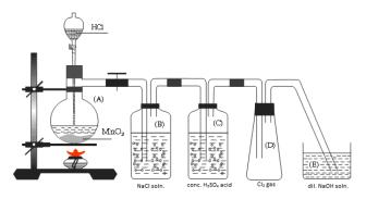
Figure 4. The apparatus was used to prepare and collect chlorine gas
