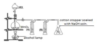
Figure 1. Collecting pure chlorine gas
