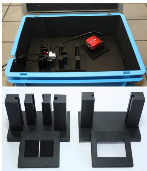
Figure 1. Spectrometer setup (top) with the essential slit, sample department and diffraction grating parts (bottom)
