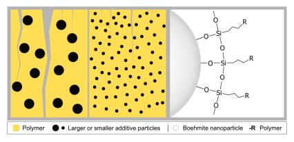
**Figure 1.** Model representation of the distribution of additives with larger and smaller particle diameters within a polymer with comparative representation of crack formation and propagation (left). Covalent between nanoparticle and polymer through functionalized surfaces (right)
