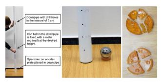
**Figure 5.** Simple characterization method (left); broken polymer and nanocomposite samples (right).
