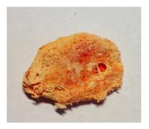
Figure 10. Precipitate 2 - Styrene-acrylonitrile
