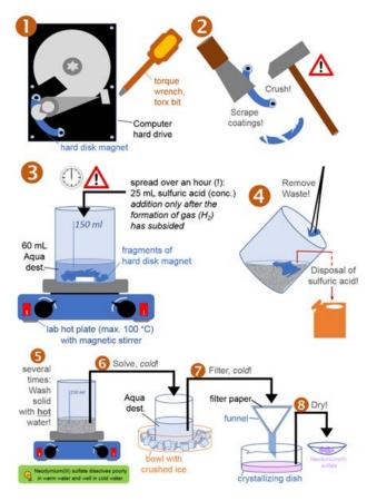
Figure 11. Experimental setup "recycling of neodymium(III) sulfate from hard disk magnets"
