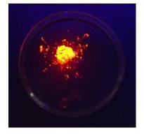
Figure 6. Luminescence of [Eu(DBM)<sub>4</sub>TEA] under UV light
