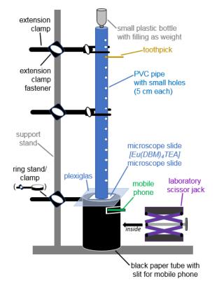
Figure 9. Experimental setup "damage monitoring"
