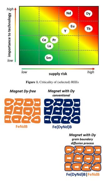
Figure 2. Schematic concept: reduction of dysprosium concentration in permanent magnet
