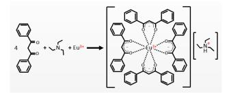
Figure 8. Chemical equation for the synthesis of [Eu(DBM)<sub>4</sub>TEA]
