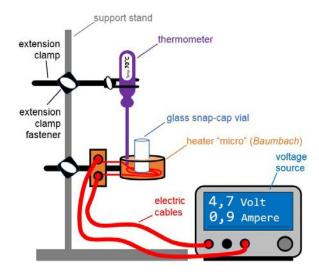
Figure 4. Experimental setup with heater "micro" (Baumbach)
