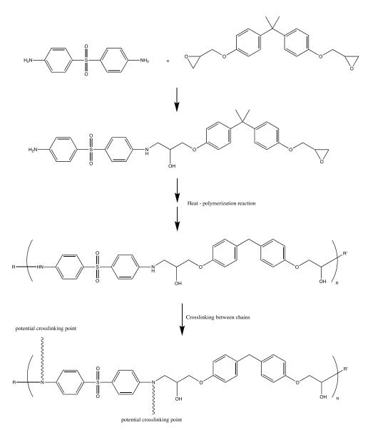
Figure B1. The reaction for the synthesis of the crosslinked epoxy resin.
