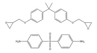
**Figure 1.** The structures of the monomers: diglycidyl ether of bisphenol A (top) and 4,4'-diaminodiphenylsulfone (bottom)
