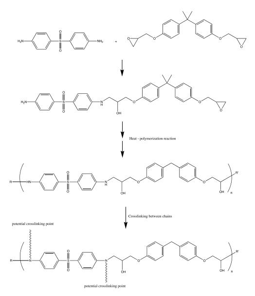
Figure A1. The reaction for the synthesis of the crosslinked epoxy resin.
