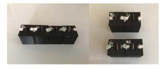
Figure 15. 3D-printed Low Cost half-cells for a pupil-centered experiment
