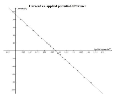
Figure 1. Cell with thermodynamic reversible electrode reactions (Measurements on the cell: Zn | ZnCl<sub>2</sub> (1 M) | KCl (1 M) | CuCl<sub>2</sub> (1 M) | Cu
