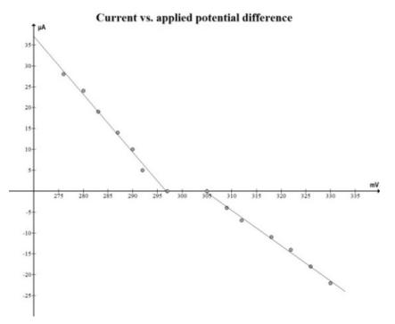
Figure 2. Cell with thermodynamic non-reversible electrode reactions (Measurements on the cell: Pb | Pb(NO\_3)<sub>2</sub>(1 M) || KNO\_3(1M) || Ni(NO\_3)<sub>2</sub>(1 M) || Ni)
