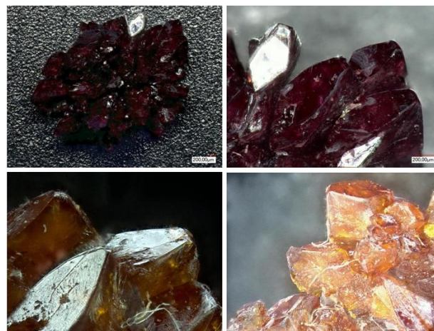
Figure 1. Spiropyran crystals under a light microscope. Top left, 50x magnification after crystallization, top right 150x magnification. Bottom left at 200x magnification after a few hours under daylight, bottom right at 100x magnification. The reddish color (top) gives way to a yellow-golden color (bottom) [15]
