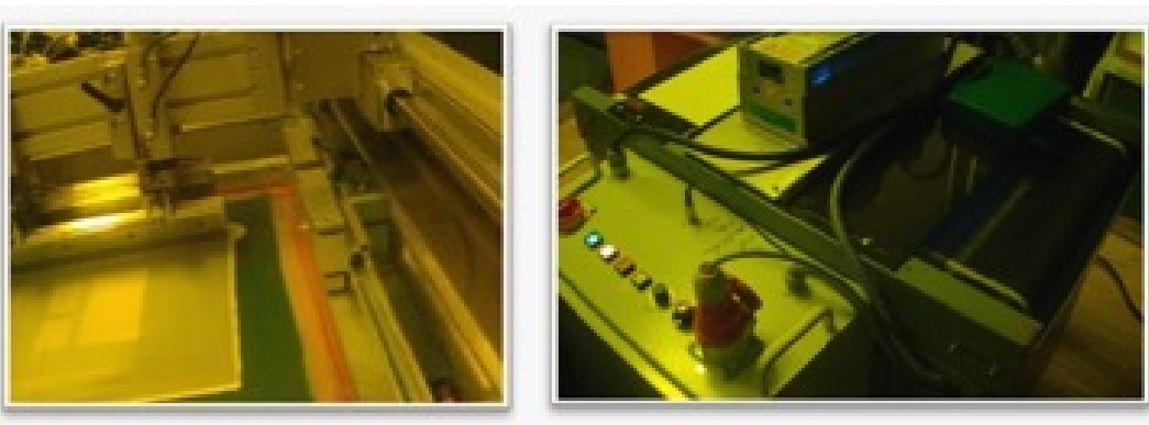
Figure 3. Screen-printer with rubber blade during printing process (left) and professional UV-chamber for curing (right)
