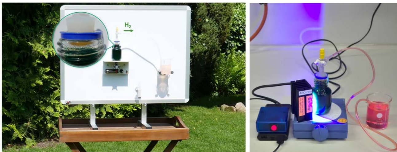
Figure 1. Setups for the photocatalytic production of hydrogen by irradiation with sunlight, and with blue light from LED. The reaction mixture is stirred magnetically, and the evolving hydrogen is pneumatically collected in a flexible tube of silicone
