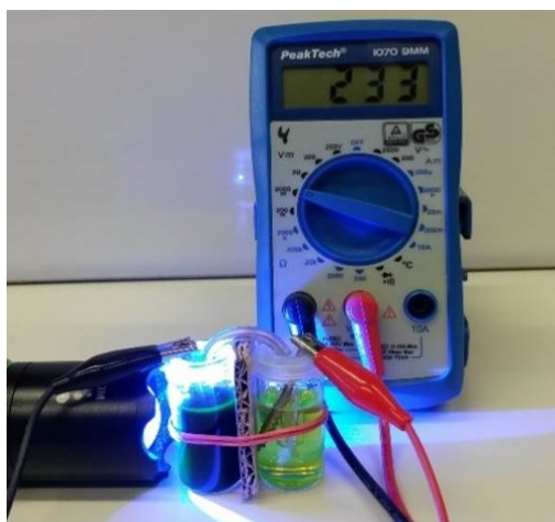
Figure 5. Concentration cell with PBB-solution in microscale version showing the occurrence of an electrical voltage by irradiation of one half cell
