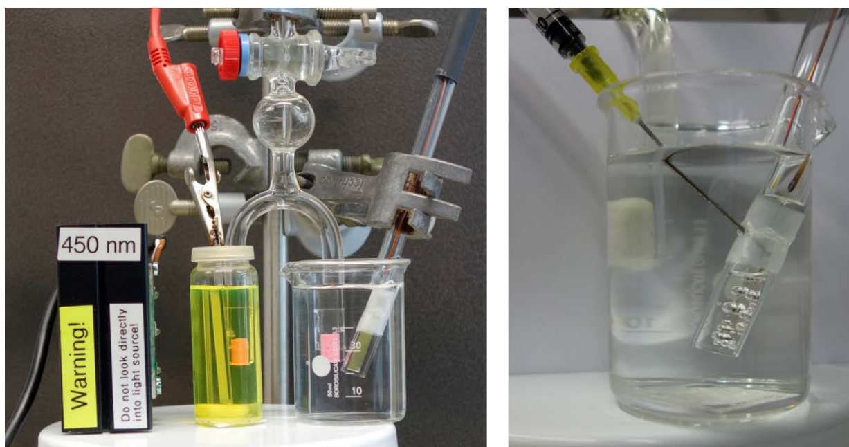
Figure 9. Photogalvanic 2-pot-cell for photocatalytic production of hydrogen, and removal of hydrogen from a sealed platinum electrode commonly used in schools
