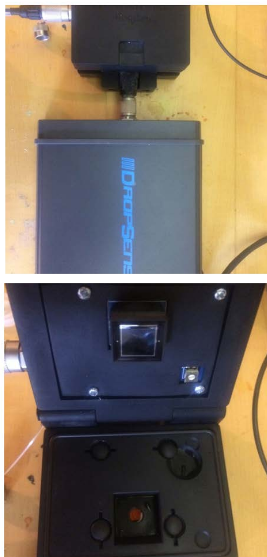
Figure 5. ECL-potentiostat (top) and ECL cell with the photodiode (bottom)
